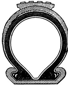
FIG. 100.—Leather-reinforced Pneumatic Tire, showing outside case of leather and spiked leather head.
